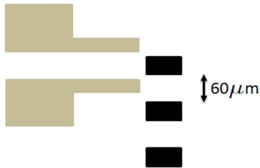
Fig. 7, Jaws specially designed to pick up objects up to 30\mu\text{m} and to pose them 60\mu\text{m} near each other.
